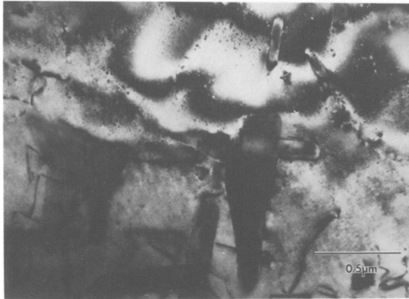
Figure 14 The Al-2 wt% Cr following 6 h at 500° C. Bright field micrograph shows coexistence of Al 7 Cr precipitates and objects of strain contrast.
